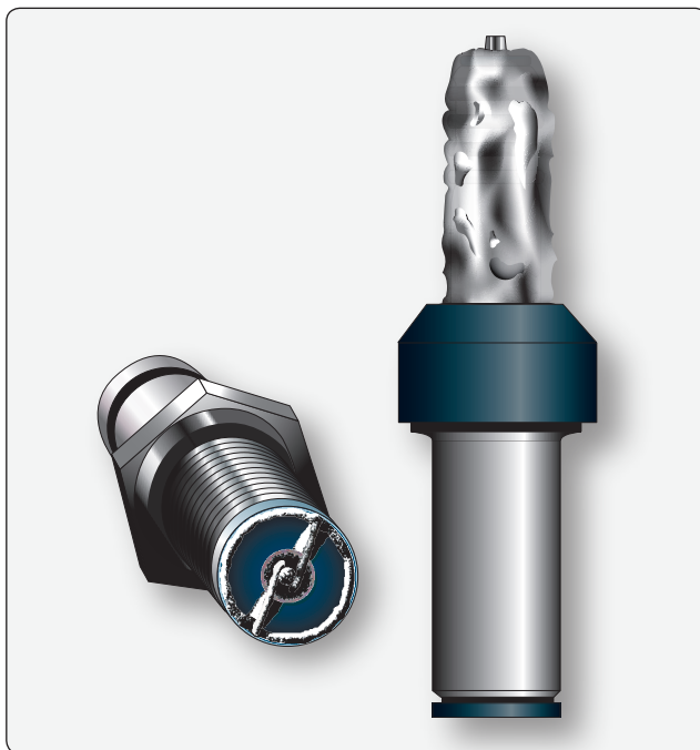
Figure 4-49. Lead fouled spark plug.
