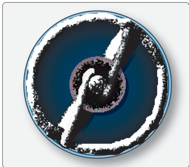
Figure 4-48. Carbon fouled spark plug.
