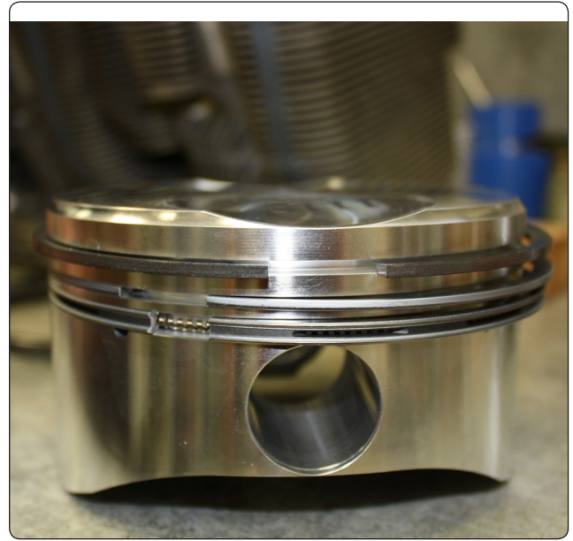
Figure 1-15. Machined rings around a piston.
