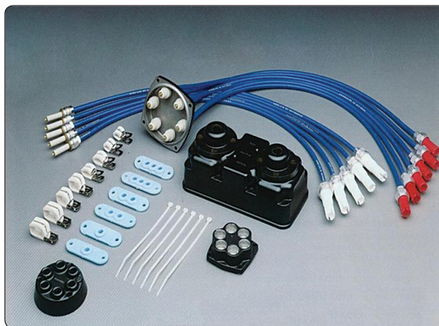
Figure 4-11. A high-tension ignition harness.
