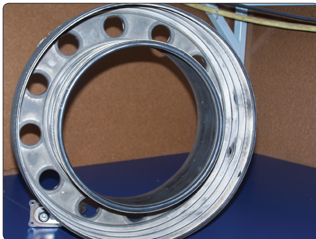
Figure 1-58. Annular combustion chamber with ceramic coating.
