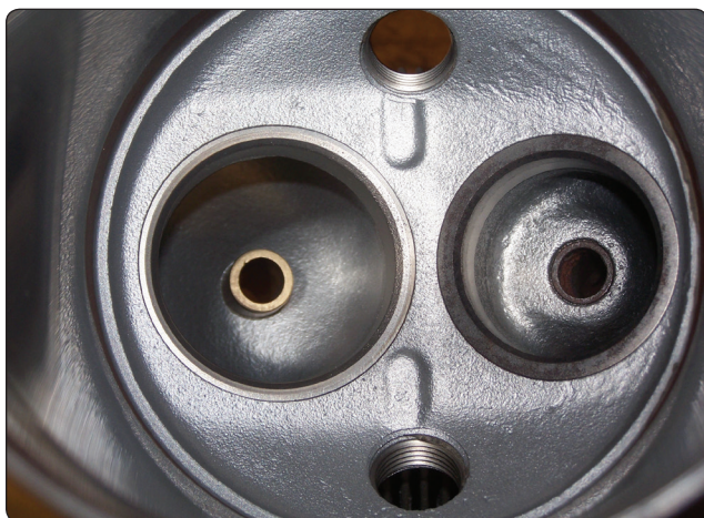
Figure 1-21. View of valve guide installed on a cylinder head.
