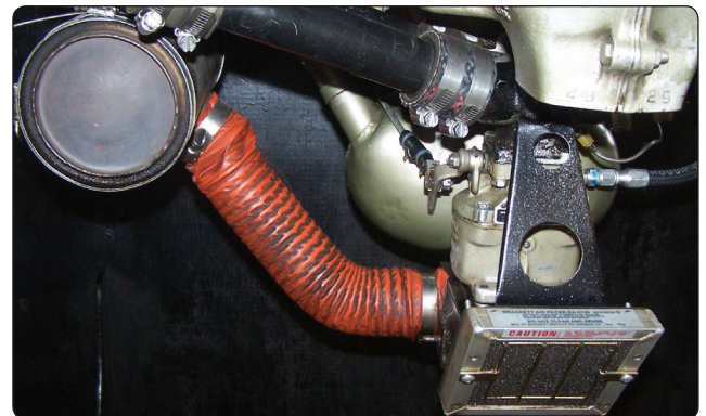
Figure 3-5. Location of a carburetor heat air valve.
