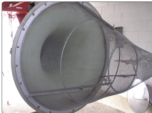
Figure 3-30. A bellmouth inlet used during system tests.
