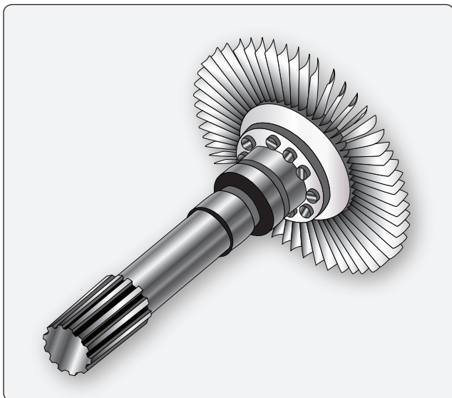
Figure 1-64. Rotor elements of the turbine assembly.
