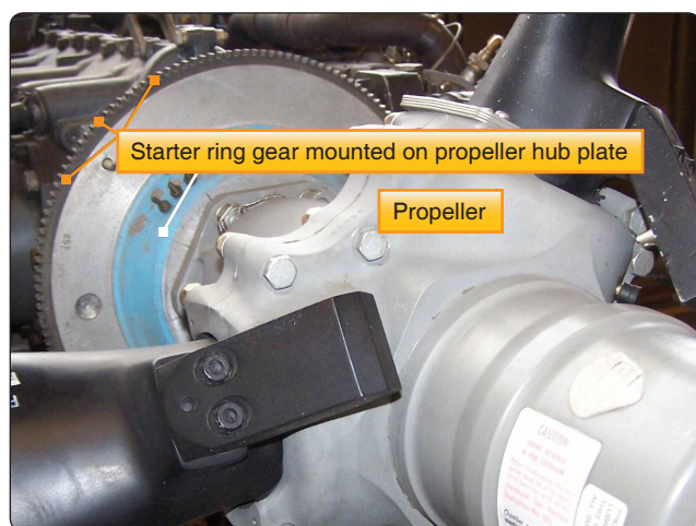
Figure 5-10. Starter ring gear mounted on the propeller hub.
