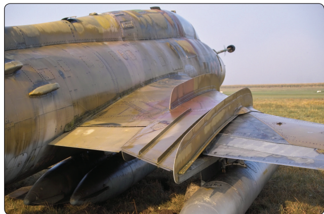
Figure 2-20. Aircraft stall fence.
