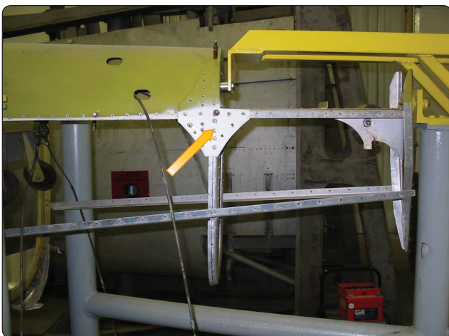
Figure 1-18. Gussets are used to increase strength.
