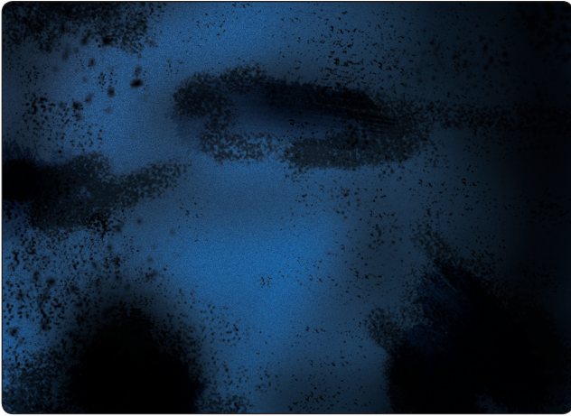
Figure 8-14. Example of blushing.
