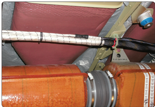
Figure 9-113. Shielded wire harness for flight control.
