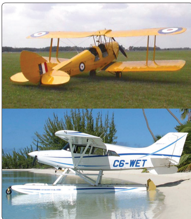
Figure 3-1. Examples of aircraft produced using fabric skin.
