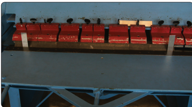
Figure 4-143. Brake alignment with two test strips bent at 90°.
