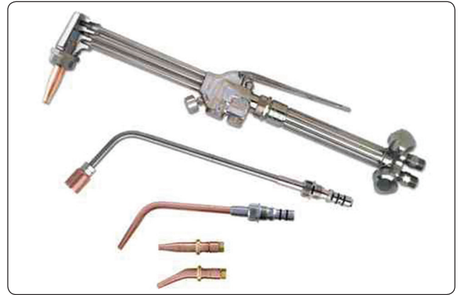
Figure 5-17. Torch handle with cutting, heating, and welding tips.
