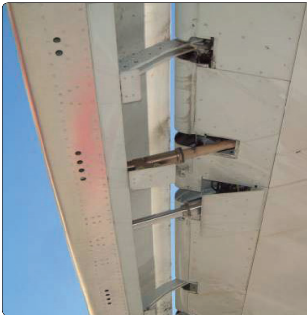
Figure 1-67. Air passing through the slot aft of the slat promotes boundary layer airflow on the upper surface at high angles of attack.
