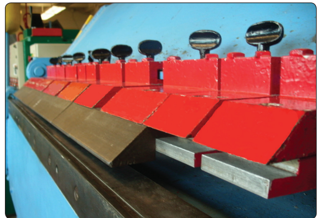
Figure 4-135. Brake radius nosepiece adjustment.
