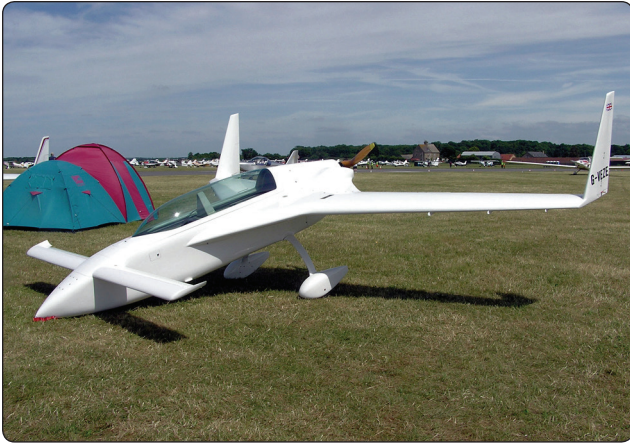
Figure 2-18. Canard wings on a Rutan VariEze.
