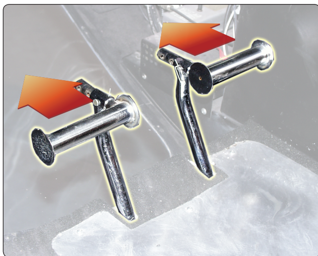
Figure 2-49. Antitorque pedals compensate for changes in torque and control heading in a hover.
