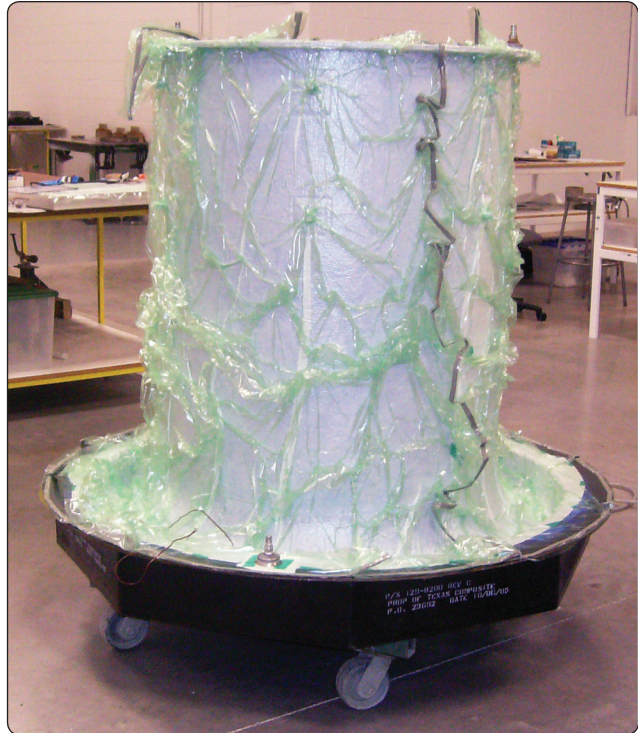
Figure 7-36. Bagging of complex part.
