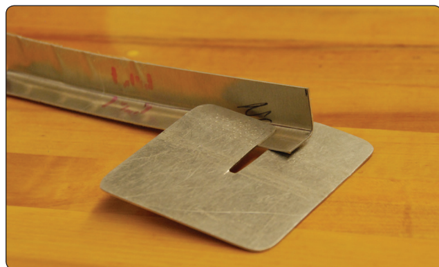
Figure 4-164. Samples of joggled metal.
