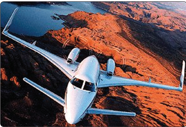
Figure 2-19. The Beechcraft 2000 Starship has canard wings.
