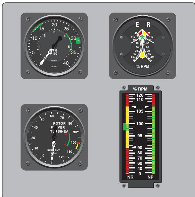
Figure 2-58. There are various types of dual-needle tachometers; however, when the needles are superimposed, or married, the ratio of the engine rpm is the same as the gear reduction ratio.
