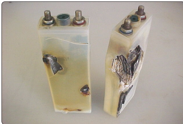
Figure 9-35. Thermal runaway damage.
