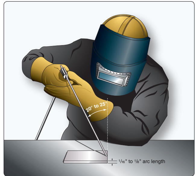
Figure 5-32. Angle of electrode.
