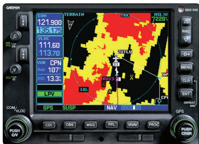
Figure 11-153. A GPS unit integrated with NAV/COM circuitry.
