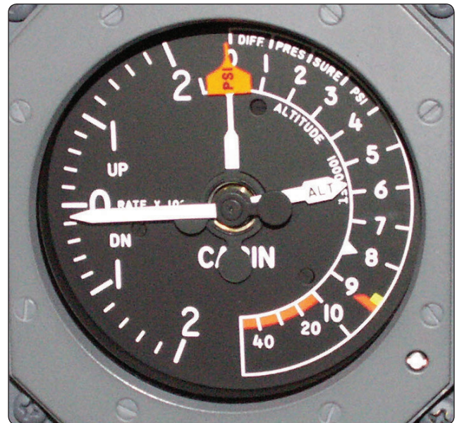
Figure 16-57. This cabin pressurization gauge is a triple combination gauge. The long pointer operates identically to a vertical speed indicator with the same familiar scale on the left side of the gauge. It indicates the rate of change of cabin pressure. The orange PSI pointer indicates the differential pressure on the right side scale. The ALT indicator uses the same scale as the PSI pointer, but it indicates cabin altitude when ALT indicator moves against it.
