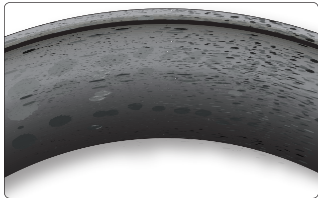
Figure 13-71. Bruising is caused by fine particle contamination possibly from a bad seal or improper maintenance of bearing cleanliness. It leaves a less than smooth surface on the bearing cup.
