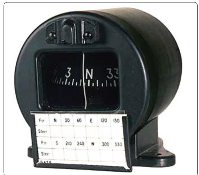
Figure 10-139. A magnetic compass with a deviation correction card attached, on which the results of swinging the compass should be recorded.
