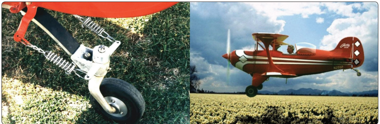
Figure 13-4. The steerable tail wheel of a Pitts Special.
