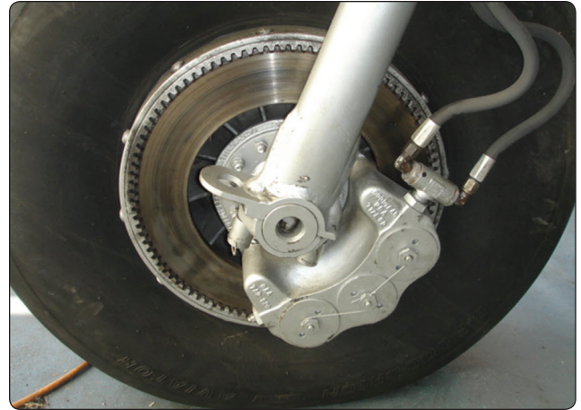
Figure 13-78. A single disc brake is a floating-disc, fixed caliper brake.
