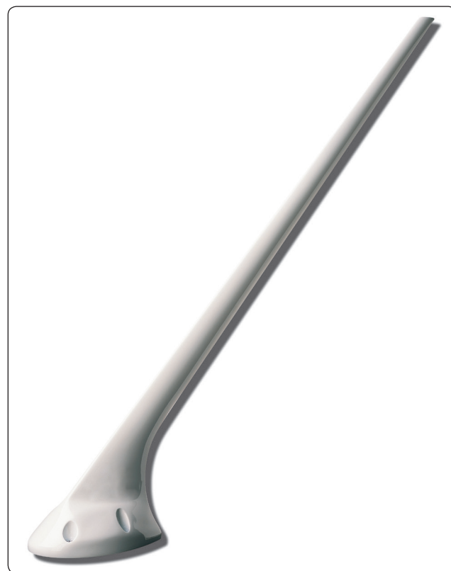
Figure 11-90. Many antenna are canted for better reception.
