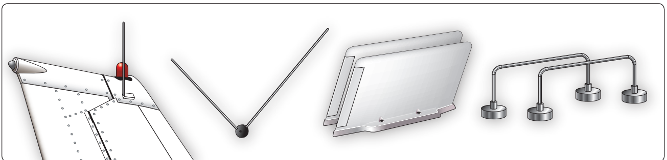
Figure 11-96. V-shaped, horizontally polarized, bi-pole antennas are commonly used for VOR and VOR/glideslope reception. All antenna shown are VOR/glideslope antenna.
