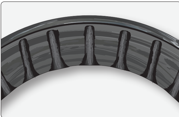
Figure 13-69. Staining and surface marks on the bearing cup that are grayish black streaks with the same spacing as the rollers are caused by water that has gotten into the bearing. It is the first stage of deeper corrosion that will follow.
