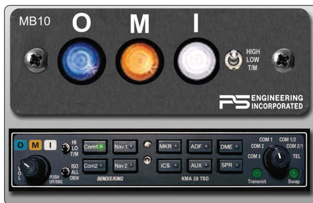
Figure 11-116. Various marker beacon instrument panel display lights.
