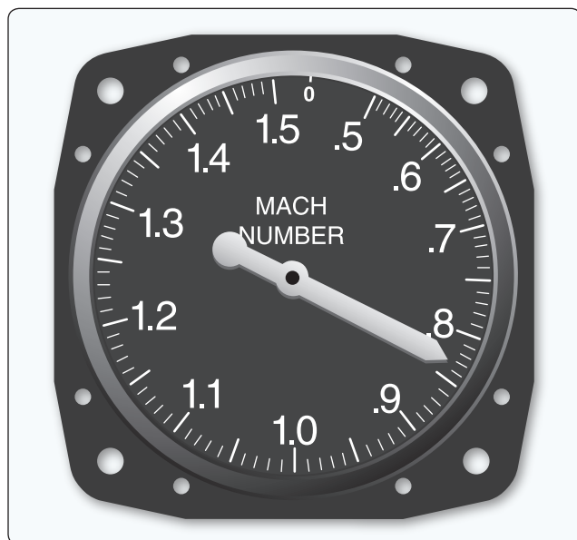
Figure 10-45. A Machmeter indicates aircraft speed relative to the speed of sound.
