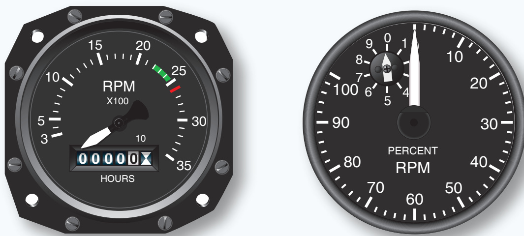
Figure 10-52. A tachometer for a reciprocating engine is calibrated in rpm. A tachometer for a turbine engine is calculated in percent of rpm.
