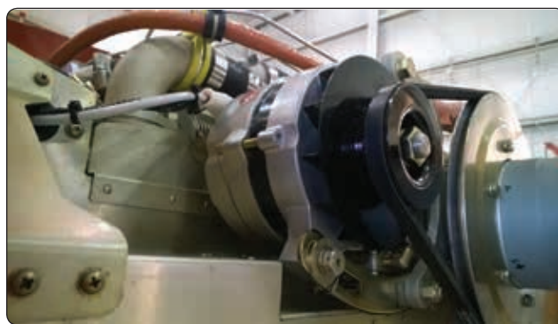
Figure 12-317. Belt driven alternator for small single engine aircraft.
