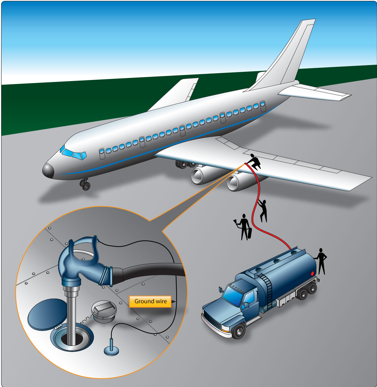
Figure 1-32. Refueling an aircraft by the over-the-wing method.
