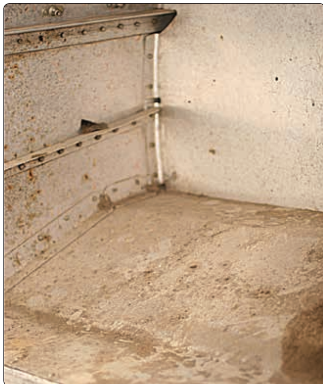
Figure 8-4. Direct chemical attack in a battery compartment.
