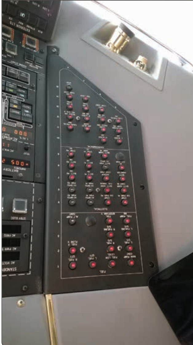
Figure 12-69. Circuit breaker assembly for aircraft electrical system.
