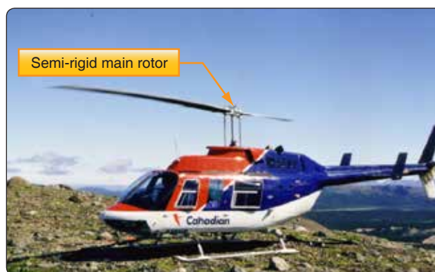
Figure 5-84. Bell Jet Ranger with semi-rigid main rotor.
