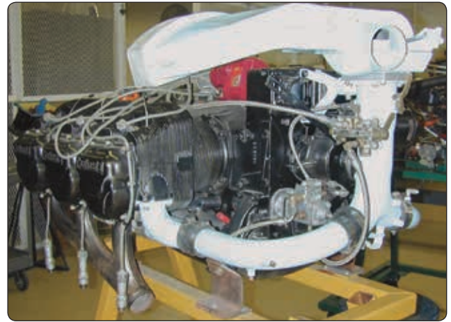
Figure 5-29. Aircraft piston engine cooled by convection.
