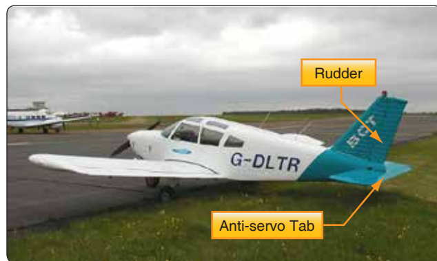
Figure 5-70. Rudder and anti-servo tab on a Piper Cherokee Arrow.
