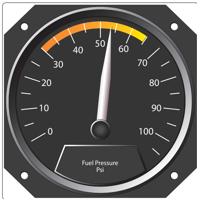
Figure 5-34. Psig read on a fuel pressure gauge.
