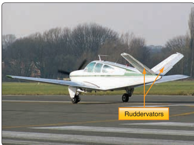
Figure 5-67. Ruddervators on a Beechcraft Bonanza provide pitch control.
