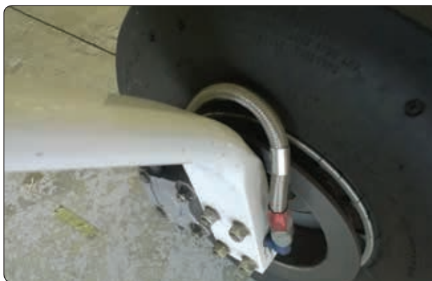
Figure 9-32. Flexible hose with stainless braid.
