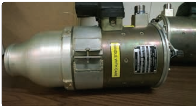
Figure 12-325. Starter generator for small business jet.
