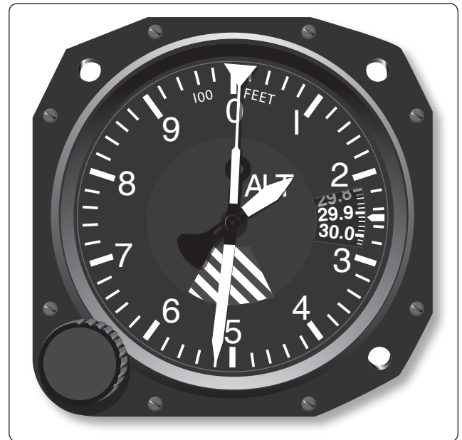
Figure 5-51. An airplane's altimeter is an aneroid barometer.
