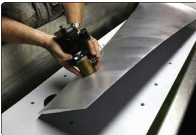
Figure 10-25. Ultrasonic inspection of a composite structure.
