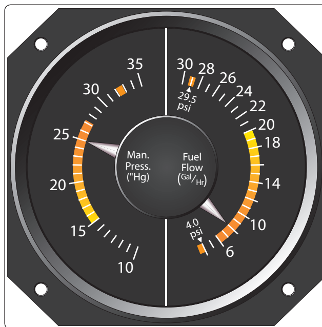
Figure 5-35. Manifold pressure gauge indicating absolute pressure.
