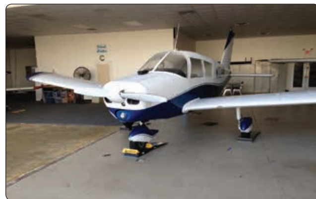
Figure 6-17. Weighing a Piper Archer using electronic platform scales.
