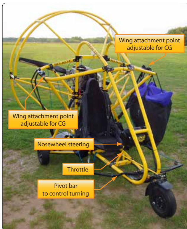
Figure 6-53. Powered parachute structure with wing attachment points.
