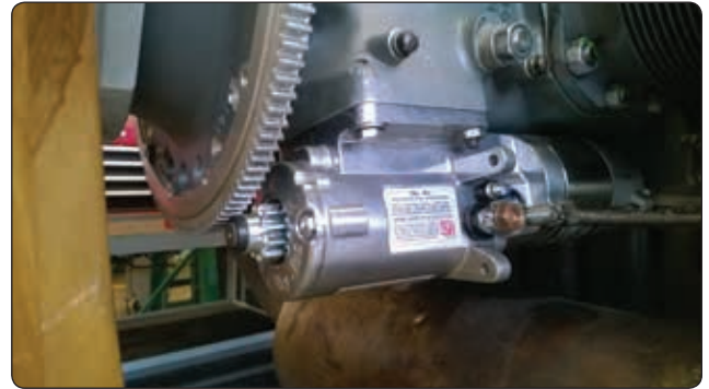
Figure 12-290. DC series starter motor.
