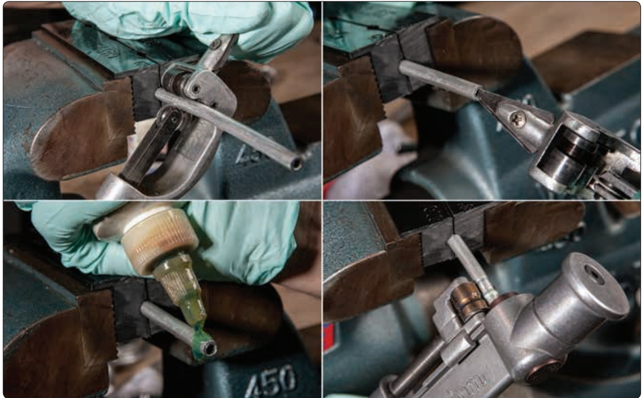
Figure 9-15. To use the hand beading tool, cut with tube cutter (1), deburr (2), oil (3), and revolve tool around tube while tightening handle (4).
