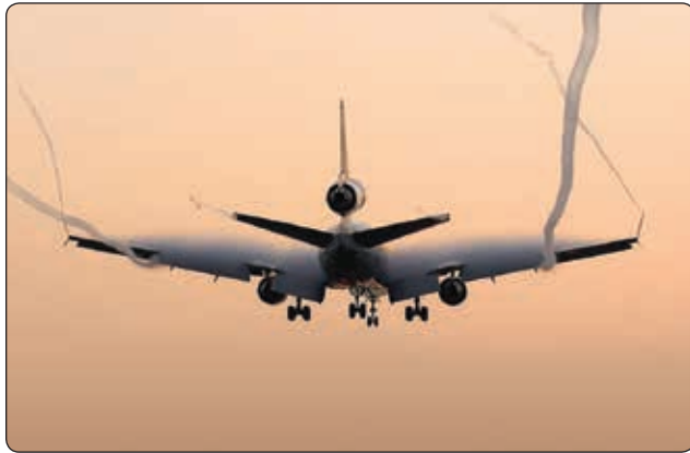
Figure 5-59. Wing and horizontal stabilizer vortices on an MD-11.
