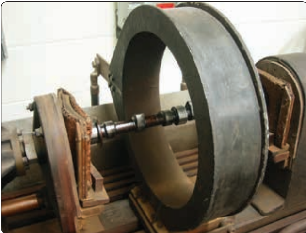
Figure 10-30. Longitudinal magnetization of camshaft (solenoid method).
