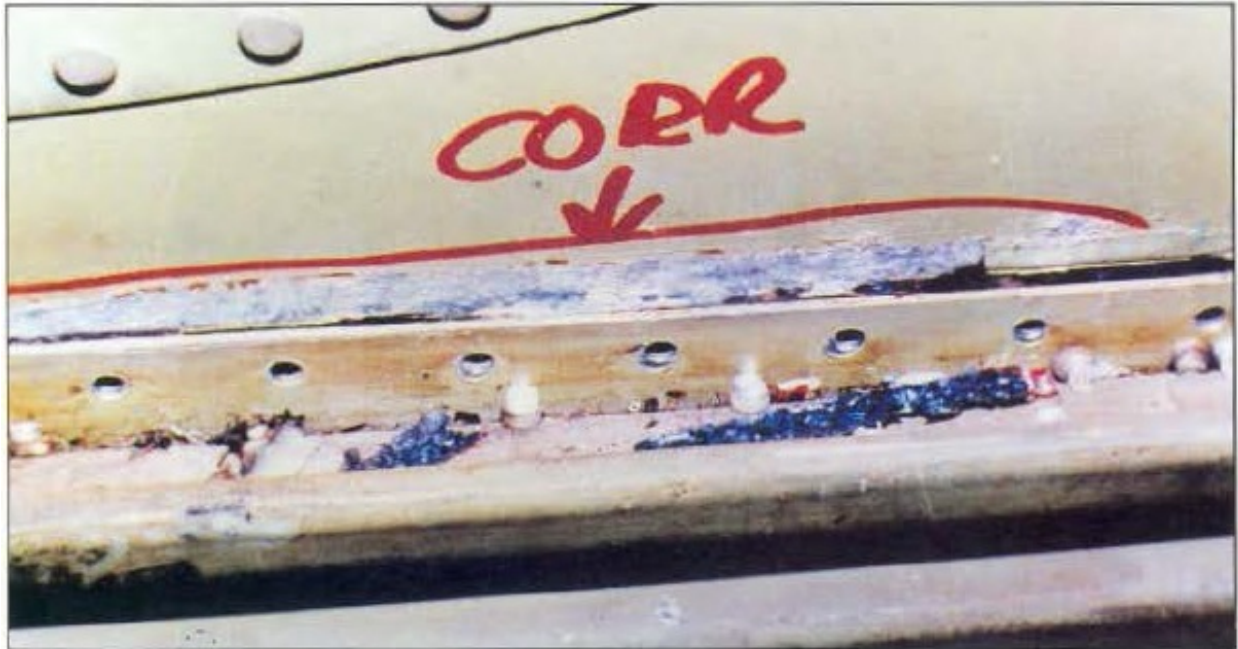
Figure 5-11. Removal of Insulation Blankets Exposed Corrosion
