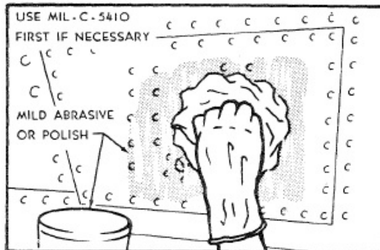
Figure 6-12. Polishing and Brightening Alclad Surfaces
